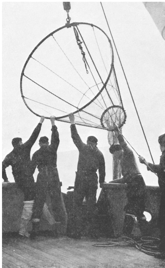
The high-speed net used to catch krill. (National Institute of Oceanography library)
